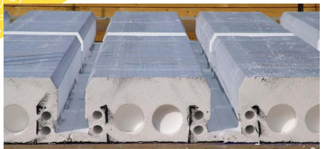
It is possible furthermore, to optimize slab thicknesses as the installations can be all fitted inside the panel longitudinal holes, thus reducing the floor intrados thickness to the bare minimum.
